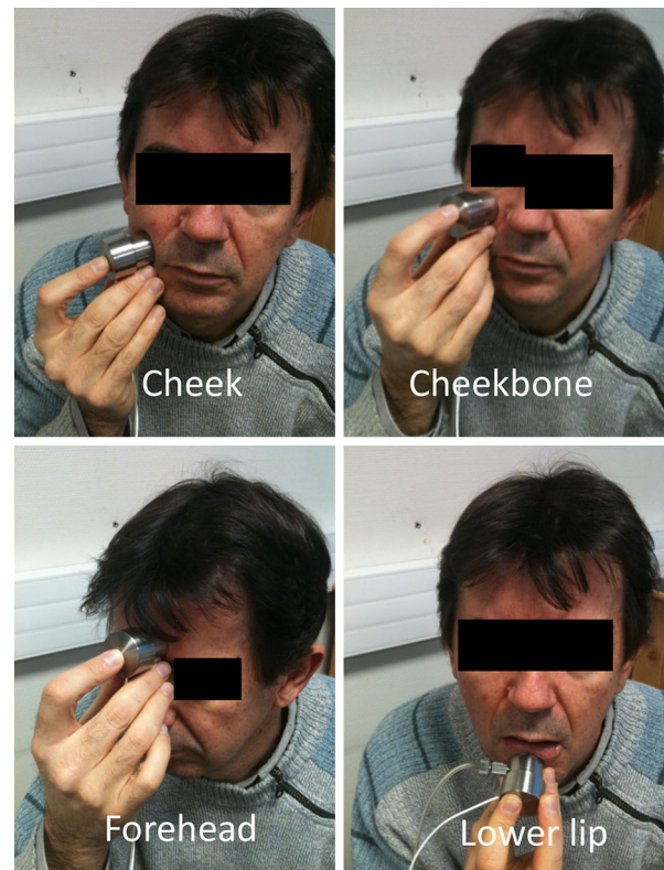
FIGURE 3. The measurements are done at four locations: the cheek, the cheekbone, the forehead, and the lower lip. The subjects are asked to position and hold LASTIC themselves under supervision of the experimenter. From the LASTIC measurements, the stiffness of the facial soft tissues at the different location can be estimated.
